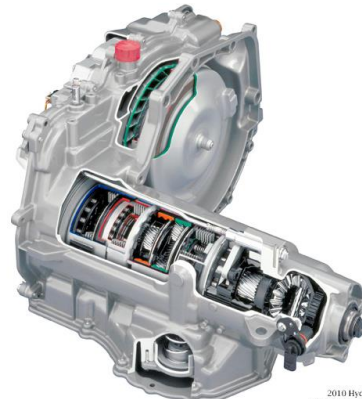
GE Hydra-Matic 4T45 FWD Fluid coupling drives 3 planetary trains plus brakes and clutches
