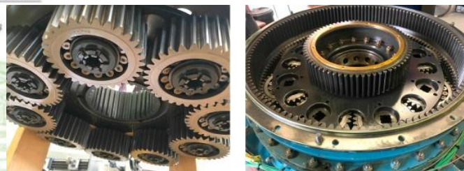
(a) 2 nd Planetary gears/ bearings (b) 2 nd Epicyclic module ring and sun gears
